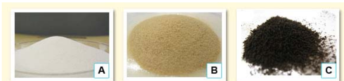
Fig. 1. Characteristics of Neusilin® US2 (A); Colloidal silicon dioxide(B) and Micronized silicon dioxide (C) grades after loading 30% oil diluted in alcohol and drying at 50°C overnight. Neusilin® showed excellent flow properties and did not show any browning or charring when compared to Colloidal silicon dioxide and Micronized silicon dioxide grades. Also, please note the electrostatic charges generated with Colloidal silicon dioxide and Micronized silicon dioxide grades.
